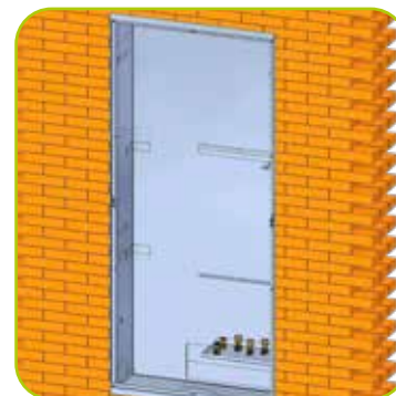
Positioning of the recessed cabinet in the wall
